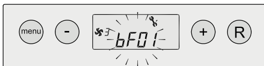
Vergrendelende storing; ventilator storing Storingsweergave knippert
